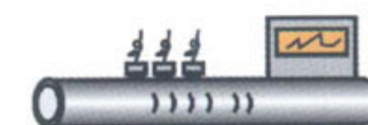
21. Eelding Seam Ultrasonic Test(UT) on the Pipe Body, Pipe-end
