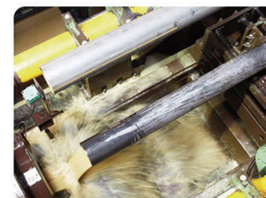
Hydrostatic testing machine With plc touch screen operating system, could print-out testing pressure automatically. it features simple construction, strong bearing member, high productivity, wide product specification range, and adjustable testing head, making it suitable for testing pressures on steel tubes of various lengths.
