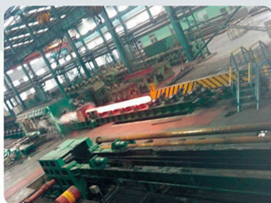
Slight-tensioned reducing mill Respective-power-transmission of three rollers ,flexible adjustment, char-artenize as high-precised of outer -diameter and superior surface funishing
