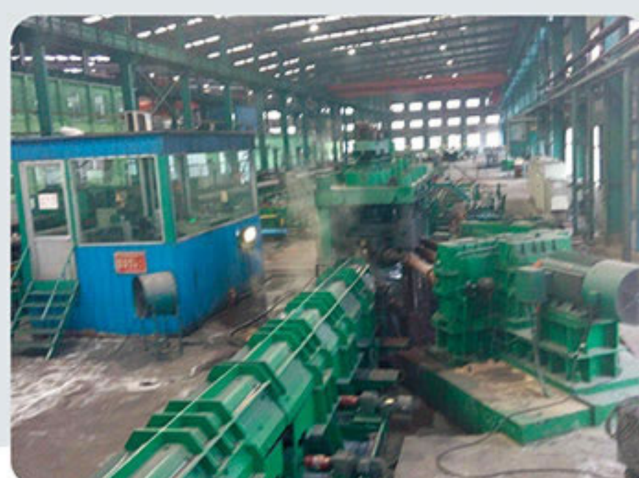
Straightener Six trollers ,eight columns, perfect rigid ,automated presed and automated angular adjustment, hydralic lock system , features as easil and flexibly operating and high precision
