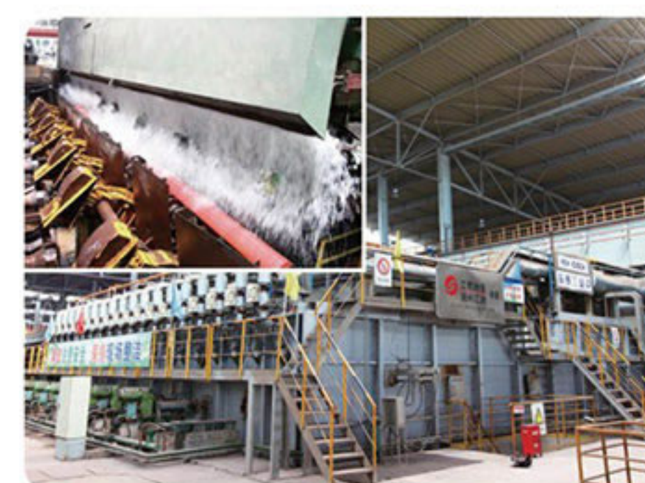
Production line advantages: Walking beam furnace with its hearth longitudinal division and horizontal, partition, the furnace temperature is automatically controlled in each section, with even temperature, so the performance properties are uniform and stable. we use water quenching with outside pouring and inside spraying. Water flowing rate and pressure can be adjusted within a large range to meet different material and different size cooling requirement. The pipes have good surface condition and precise dimension after high pressure water descaling and hot sizing. Supporting equipment: Walking beam quenching furnace, Walking beam tempering furnace, UT&EMI combination test machine from GE & FOERSTER, Six-rollers straightener from BRONX
