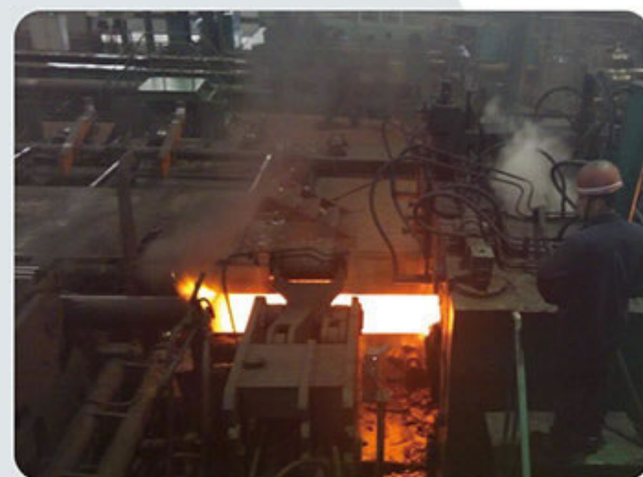
Accu-rolling mill Conical Roller ,big disk,flexible adjustment,hydraulic-controlled lock system and balance system ,easy and reliable operation
