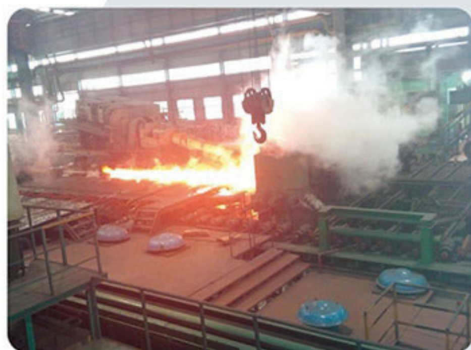
Piercing mill The punching machine can be adjusted automatically and locked hydraulically , this unit features in stable punching process, uniform hair canal wall thickness etc.This Machine is advanced at home.
