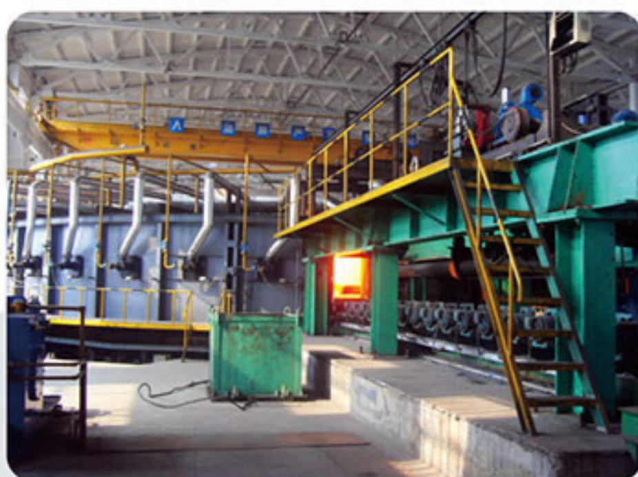
Rotating heat furnace Single-or dual-feeding available ,fueled by lpg, automated furnace- temperature. Furnace-pressure and furnace flow ,domestical-topping controlling performance
