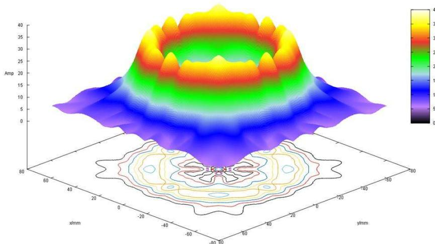
Figure 2. A representative sound field generated by the ShapeUT™ function in  $360^\circ$
