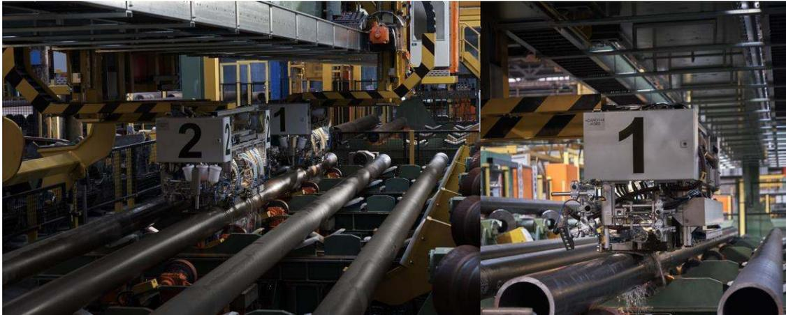
**Figure 4. The installed 2D-matrix UT-machine at the Vallourec mill in the Düsseldorf-Rath, Germany.**
