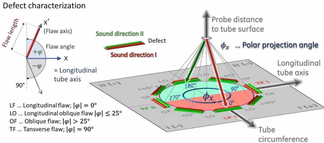
Figure 1. Defect characterization including the definition of the defect orientation
