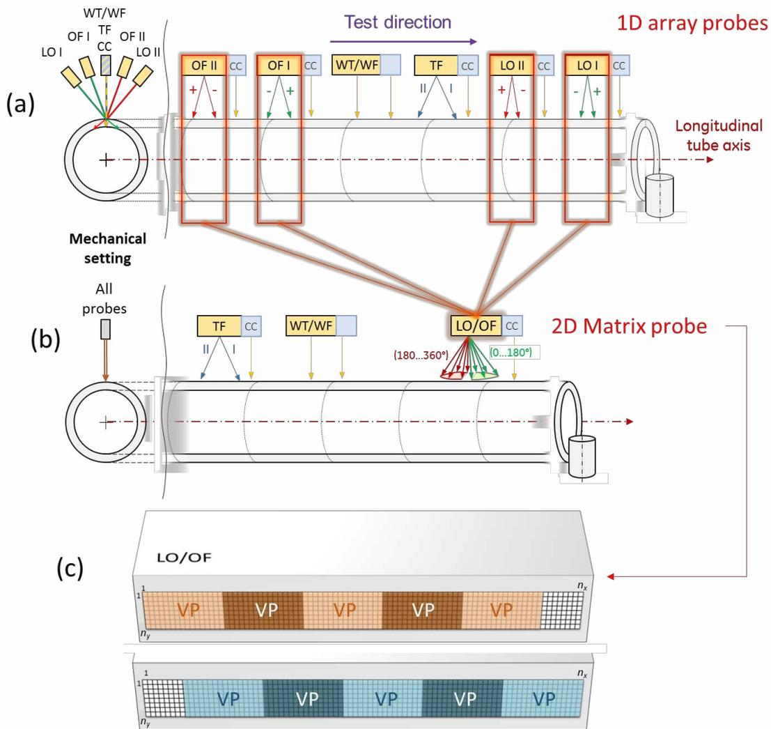
**Figure 3. State-of-the-art UT system equipped with 1D array probes (a) in comparison to the new system including a 2D matrix probe (b). Schematic sketch of a possible configuration of virtual probes (VP) is shown below (c).**
