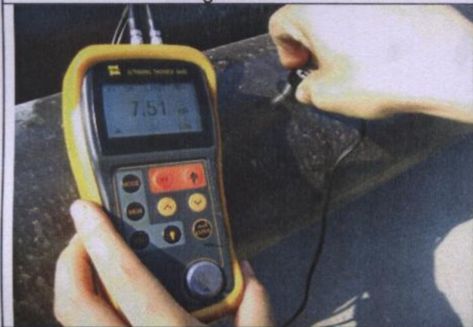
Wall thickness check
