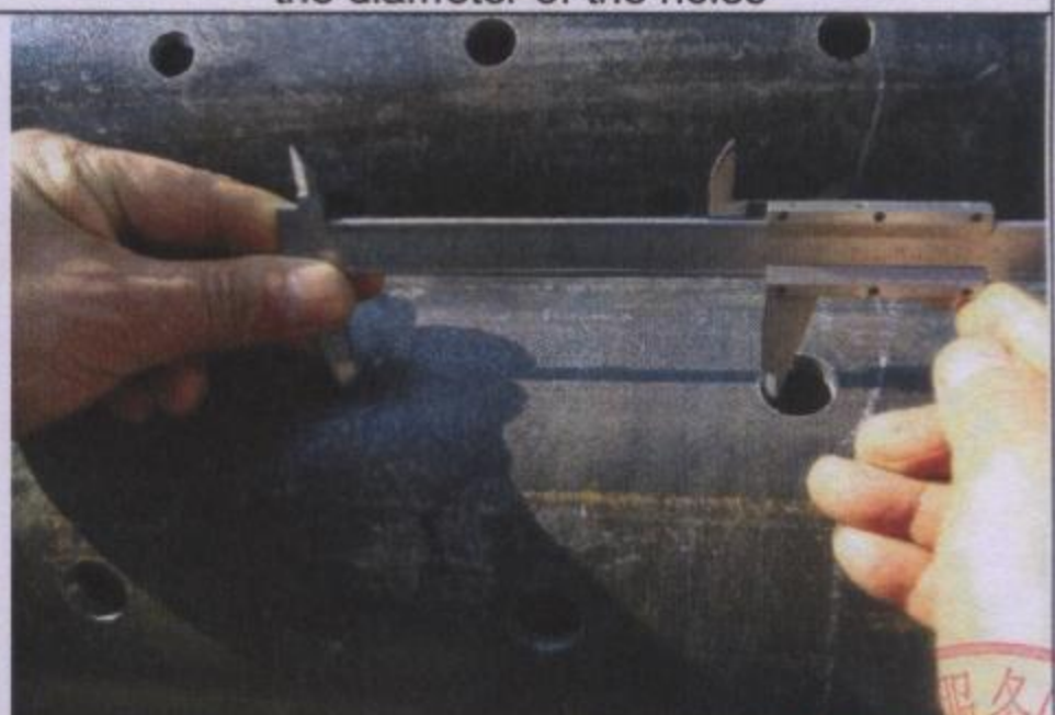
Dimension check for hole distance
