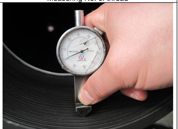
Measuring Tolerance of tooth depth
