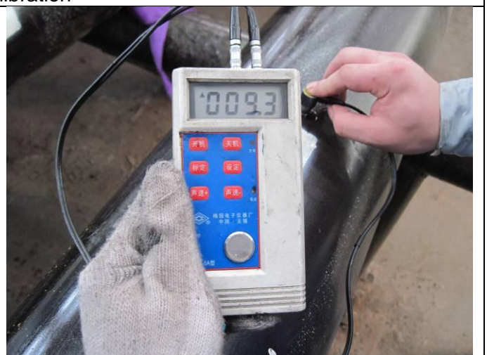
Measuring WT of pipe
