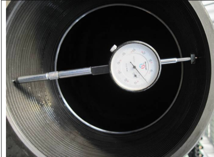
Measuring Taper of coupling thread
