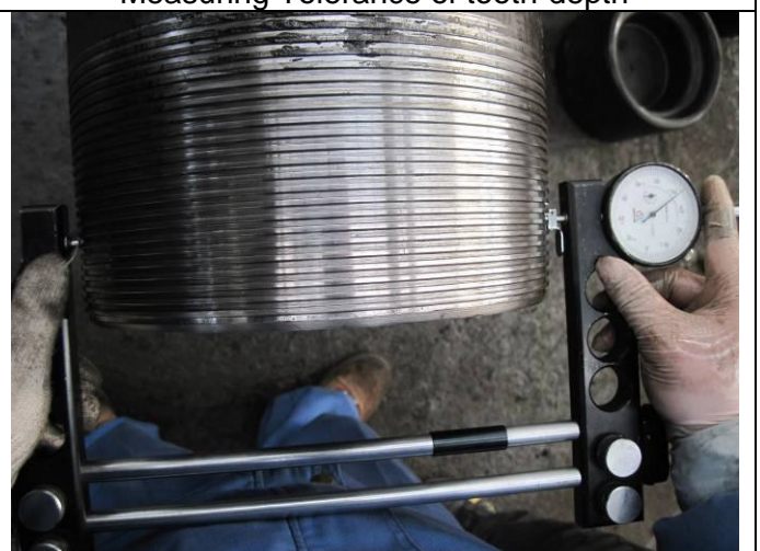
Measuring Taper of pipe thread
