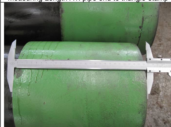
Measuring Length of coupling
