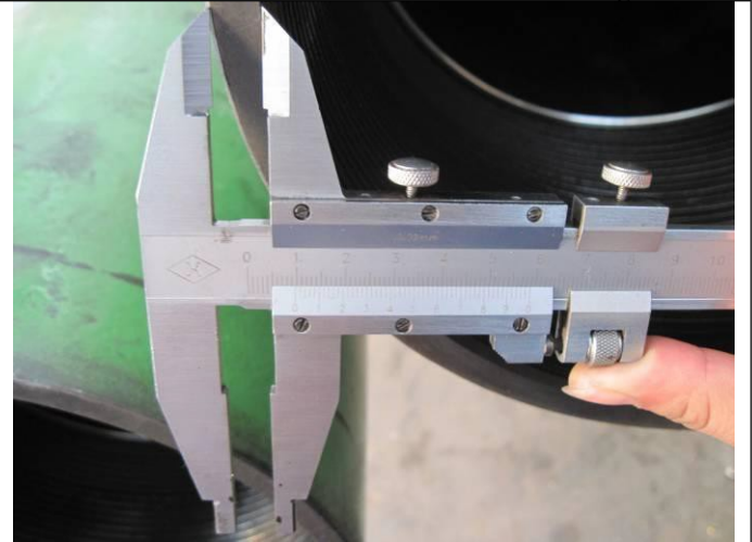
Measuring b: Width of bearing face
