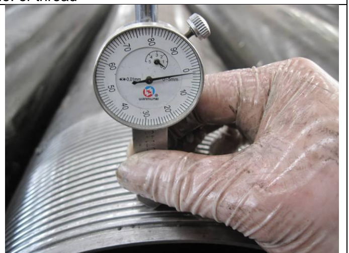
Measuring Tolerance of tooth depth
