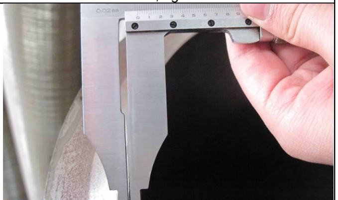
Measuring bevel angle in accordance with ASME B16.25, fig. 3a
