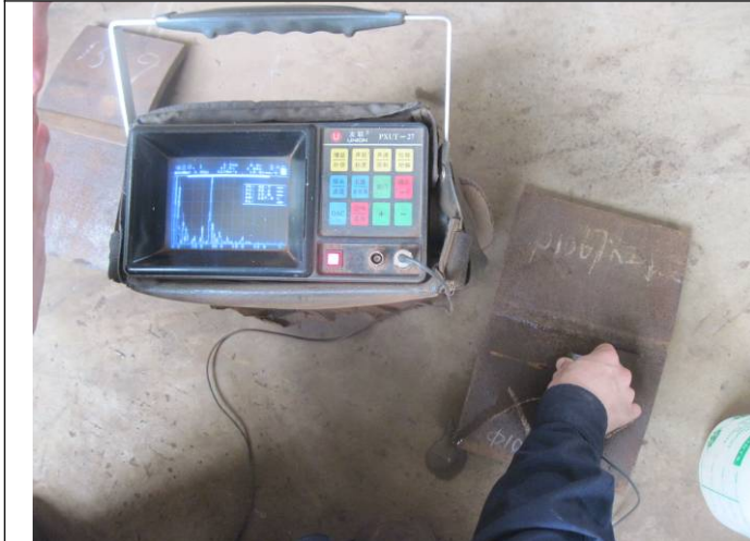
UT equipment 2 calibration
