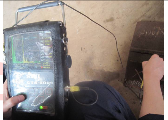
UT equipment 3 calibration
