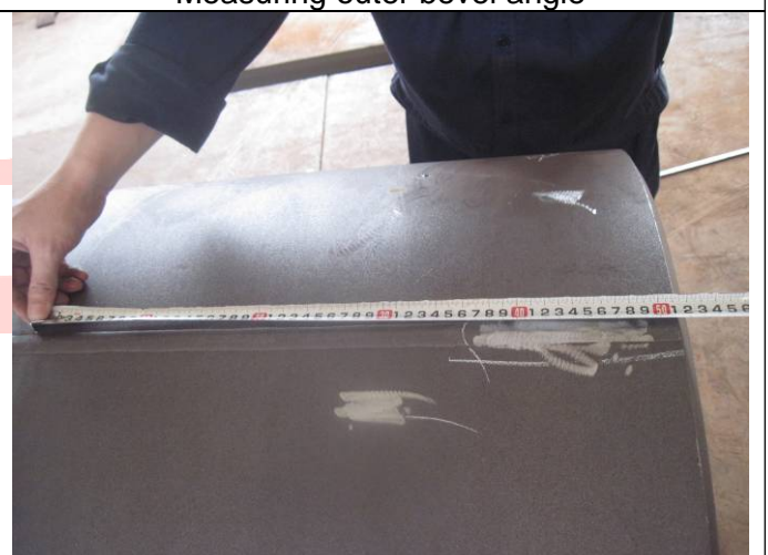
Measuring straight tangent end
