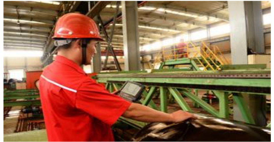
Manual Ultrasonic Flaw Detection
