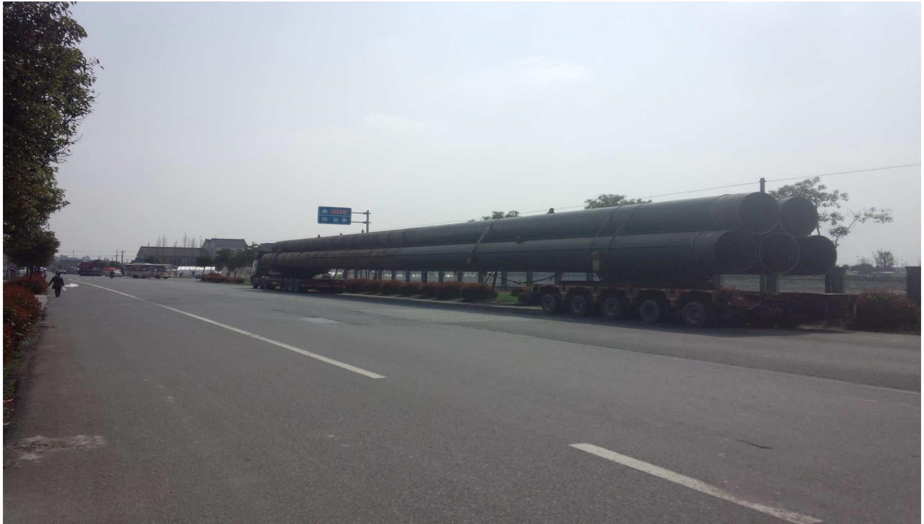
TRUCK TRANSPORTED EXTRA LENGTH PIPE PILING
