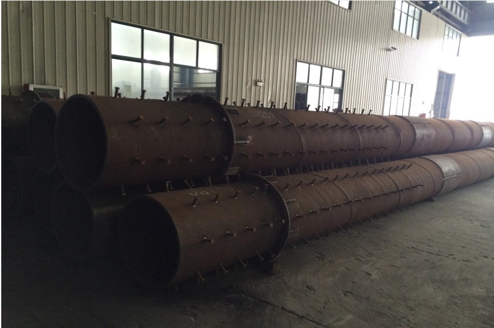
AS1163 C350L0 STUBBED PIPE PILING
