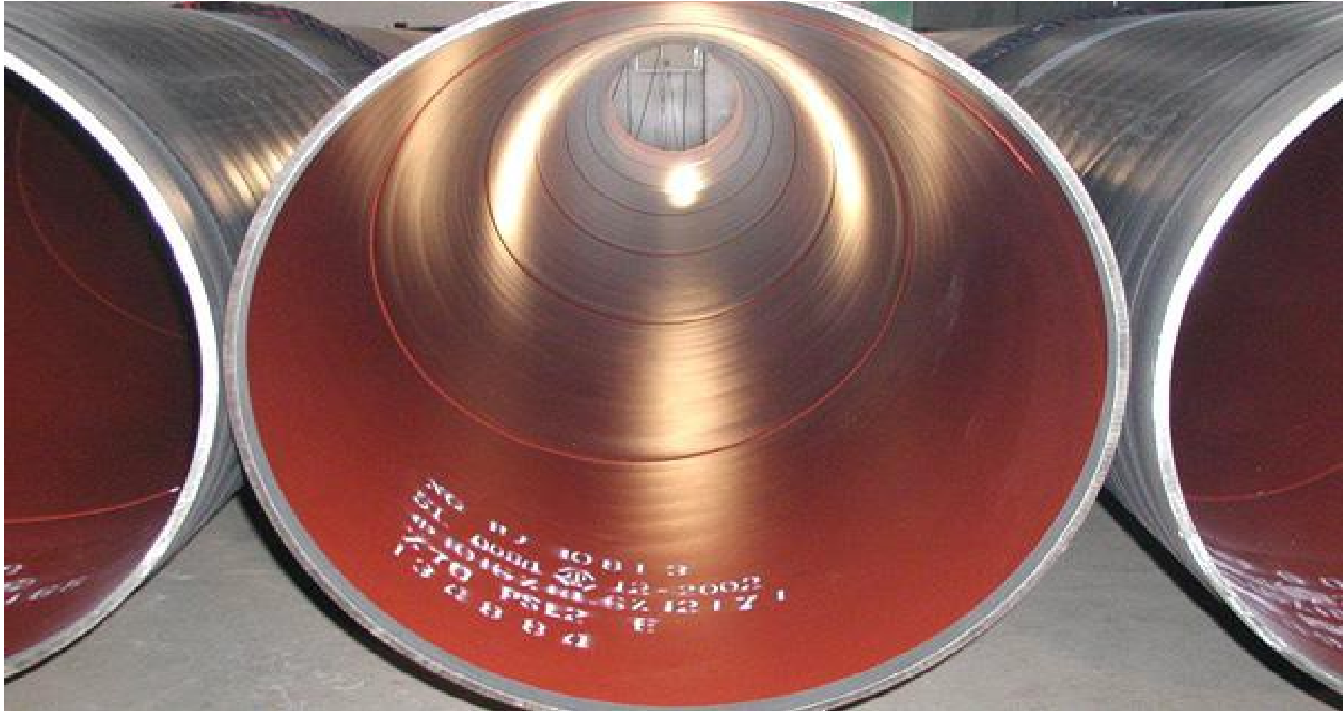
LIQUID EPOXY LINING+3LPE COATING
