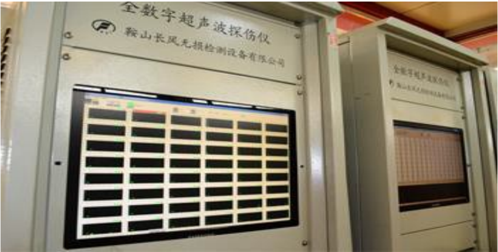
Continuous Monitoring Equipment of Ultrasonic Flaw Detection
